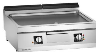
Available only for countries outside the European Community. Griddle made of AISI 304 stainless steel, 20/10 mm thickness top. Satin finished Fe510D steel cooking plate. EVEN-PRO SYSTEM. Delivered with: plate plug. Heating by two independent heating elements made in AISI 309 stainless steel placed under the plate, safety thermostat. Working temperature (min-max): 70-260°C.
